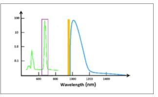
In the picture above the laser excitation is presented as yellow line and autofluorescence as blue curve. The emission signal presented as green curve can be measured free of autofluorescence.
