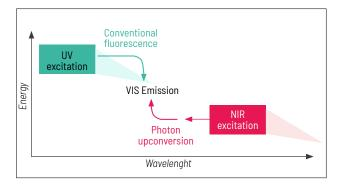
In Upcon, the label is excited at long wavelengths (NIR) and emission is detected at shorter wavelengths (VIS). Autofluorescence occurs always with longer wavelengths than excitation, so autofluorescence will not disturb the detection with visible wavelengths.
