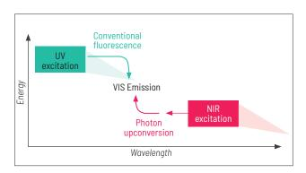
In Upcon, the label is excited at long wavelengths (NIR) and emission is detected at shorter wavelengths (VIS). Autofluorescence occurs always with longer wavelengths than excitation, so autofluorescence will not disturb the detection with visible wavelengths.
