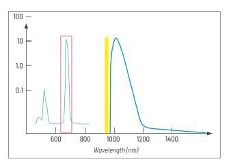
In the picture above the laser excitation is presented as yellow line and autofluorescence as blue curve. The emission signal presented as green curve can be measured free of autofluorescence.
